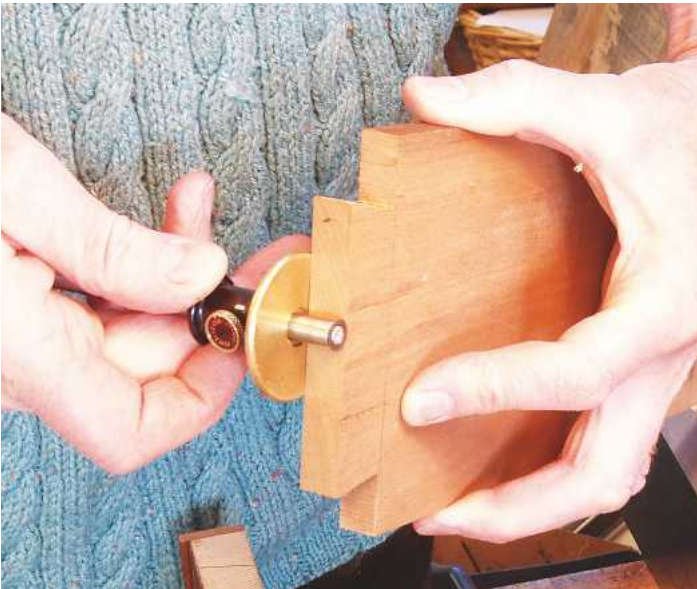
▲ Pic.8 Transferring tail board thickness to pin board
